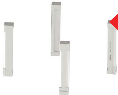
Figure 1 – The REMco IronSide design uses drop-in type tungsten tips for ease of replacement and low cost operation. Multiple grades of tungsten are readily applied for maximum wear life depending on rock type. No bolts are used to hold the tungsten tips in place.
