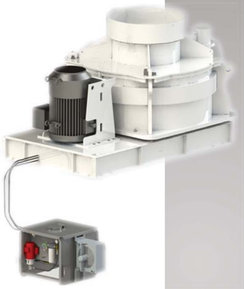
Figure 2: 3D model showing the oil system mounted lower than the crusher for gravity return of the oil.
