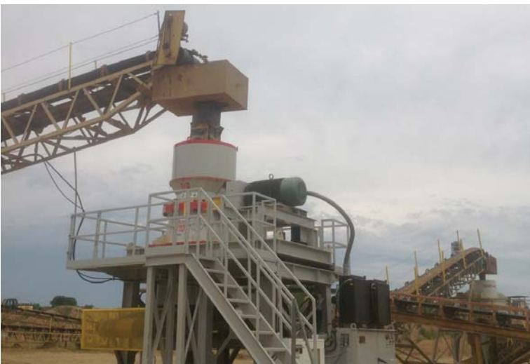
Figure 4: The REMco PROcone 4510 in operation. The PROcone is engineered with a large feed opening that remains consistent throughout the life of the manganese liners.
