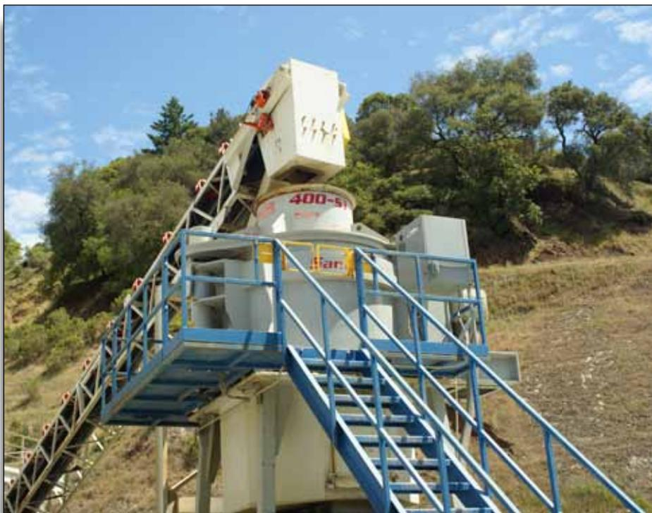
The second VSI unit is **REMco Model 400 SandMax** used to produce C-33 tight specification concrete sand with excellent FM. This machine was installed in 2009 as part of the BoDean's company expansion to meet the growing concrete demand of the Saint Helena / Santa Rosa California area. Using solar generated electric power to drive this machine, BoDean further lowers its sand production cost.
