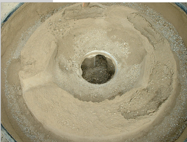
Figure 1: Extreme example of excessive build-up in the crushing chamber causing the machine to stall.
