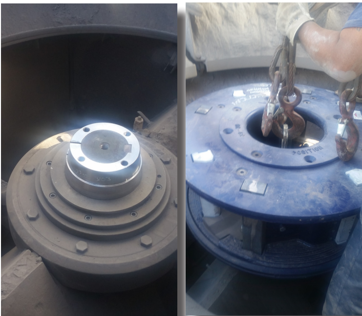
Figure 4: (left) REMco’s boss placed on the Sandvik bearing cartridge (right) 37-4-14 rotor being installed onto the bearing cartridge.
