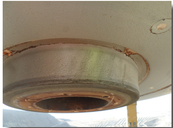
Figure 2: Example of excessive wear on the rotor boss skirt (top) versus a new rotor boss skirt (bottom).
