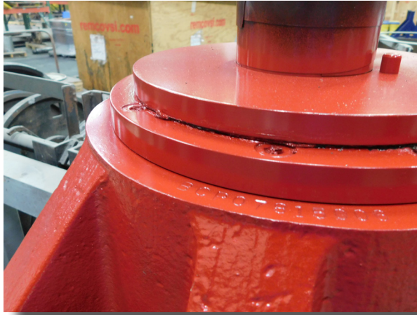
Figure 4: Example of new seal plate on bearing cartridge.
