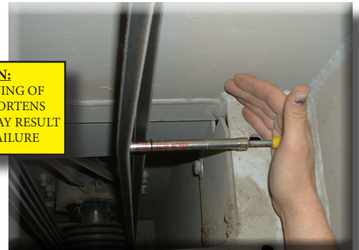
Figure 2: Using the belt tension tester to accurately determine the belt tension of the crusher.
