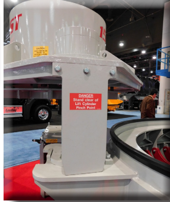
Figure 4: The hopper lid moves in either direction and the safety stop allows the operator to position the lid.
