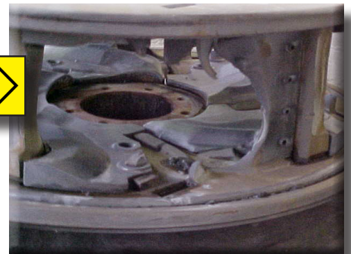
Figure 3: This was the damage created when work was done to the motor, the rotor ran backwards.
