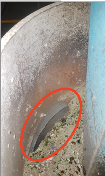
Figure 1: Customer A noticed a hole in the top of their hopper lid (left), and discovered the feed tube completely worn through, and a hole on the bottom of the hopper lid (top).
