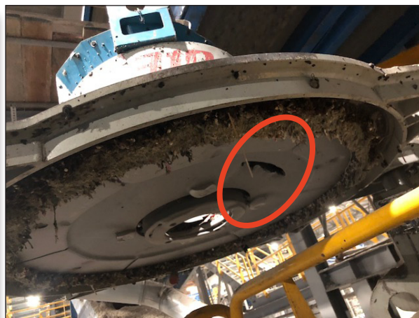
Figure 1: Customer A noticed a hole in the top of their hopper lid (left), and discovered the feed tube completely worn through, and a hole on the bottom of the hopper lid (top).
