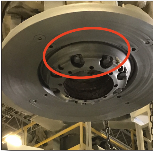
Figure 2: Customer B has worn through the rotor skirt causing material to enter into the bearing cartridge.
